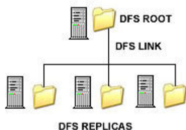
Figure 1: The actual folder structure of DFS and load balancing
